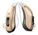
Signia Motion 13 Nx hearing aids - offer the most versatile fitting options and can be equipped with a telephone coil without significantly enlarging the housing.
